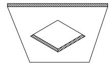
1. Open a hole as the suggested cut-out dimension on the ceiling
