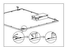
3. Bend the pre-installed clips on the luminaire
