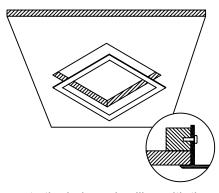
2. Fix the frame to the hole and ceiling with the supplied screws
