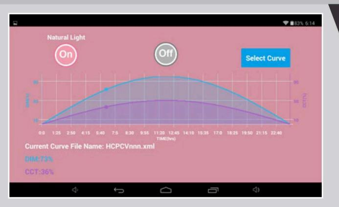
In the **Dynamic Light Mode**, the CCT and brightness of the HCP fixtures will automatically change at the times on the curves. The pre-set curve mimics the pattern of natural light over a 24 hour time frame.
