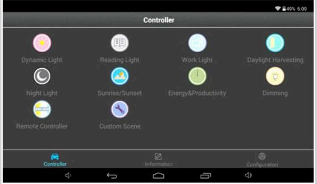
\*Each mode uses the "On and "Off" buttons to control the fixtures.
