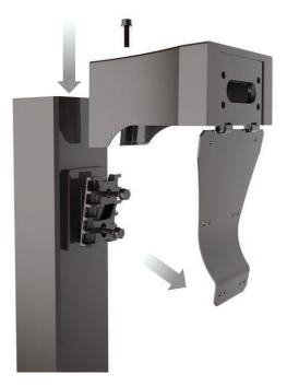
Swing-down, Hinged Arm Door convenient for wiring
