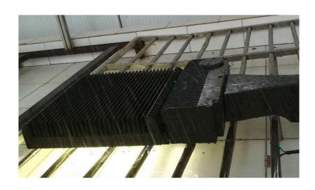
No water leakage Real IP66 rated
