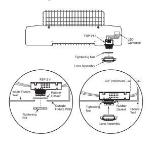
The FSP-211 accommodates fixture wall thickness up to 0.125" (3.18mm)
