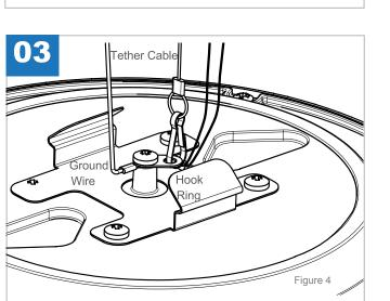
Attach the Tether Cable to Hook Ring on the back of fixture. See Figure 4.
