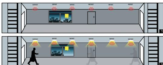
1. No motion detected, all lamps switch off.
