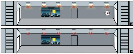
3. No motion is detected in detection area, all lamps synchronously dim to a low light level after hold time.
