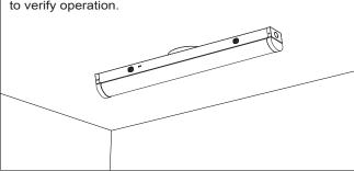
8. Swing open fixture by pushing in/squeezing both buttons located on opposite ends, if need to disassemble the fixture
