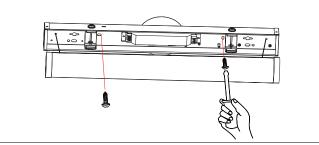
6. Press upward the cover and lock it with springs tightly which located into the fixture.
