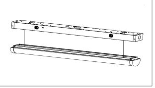
3.Run the fixture's power wires through the center hole of the round J-box adapter. Slide and secure the J-Box adapter on the center slots located on the back of the Note: J-Box adapter is used to cover the Junction Box
