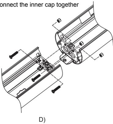
Step1: use the screw 3xUNC8-32 connect the inner end c
