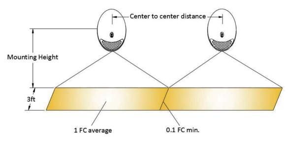
Requirements: 1.0 foot-candle average and 0.1 foot-candle minimum with a 40:1 maximum/minimum ratio. The corridor used is 80 feet long, 9 feet ceiling with a 6 feet wide walkway and 6&3 feet path of egress. The reflectance are 80% ceiling, 50% walls and 20% floors. The fixture mounting height is 7.5 feet.
