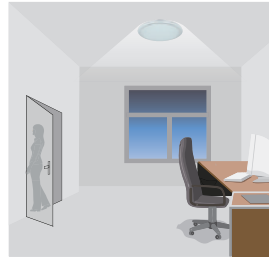
3. No motion is detected in detection area, all lamps synchronously dim to a low light level after hold time.
