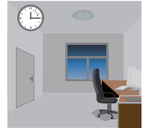
4. After stand-by period, the lamps switch off if no movement is detected in the detection zone.
