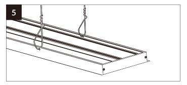
Fix the aircraft cable on the long bar
