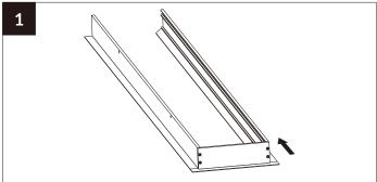
Joint the 2pcs long bars and 1pc short bar together with screws
