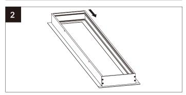
Then joint these 2pcs long bars and another short bar together with screws.
