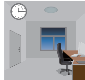
4. After stand-by period, the lamps switch off if no movement is detected in the detection zone.
