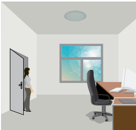
1. No motion detected, all lamps switch off.
